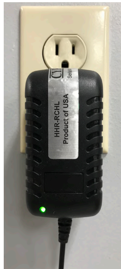
The LED is green; the reader is either charged or not in the HHR-DOCK.
