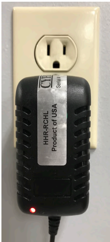
The LED is red; the reader in the HHR-DOCK is charging.
